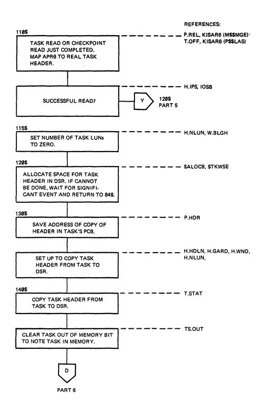
Figure 2-11 Loader Logical Flow Diagram (Part 5 of 8)
