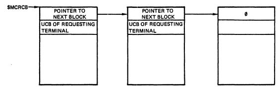
MCR queue entries in this list are dequeued when an external MCR command (a task with a taskname... XYZ) issues a GMCR\$ directive; the contents of the entry is copied into the DPB of the GMCR\$ directive and the MCR queue entry is deallocated
