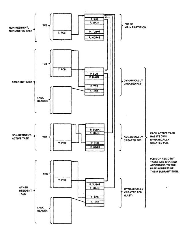
Figure 8-8 TCB, Task Header, and PCB Relationships in a System-Controlled Partition
