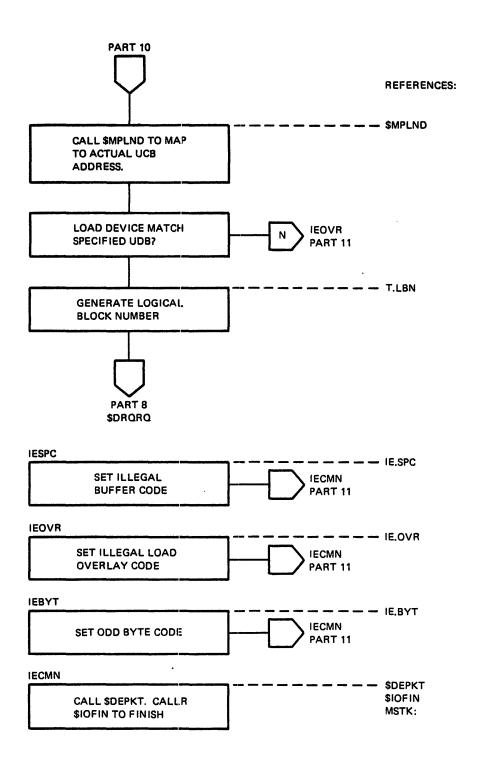
Figure 6-2 QIO Directive Processing (Part 11 of 24)
