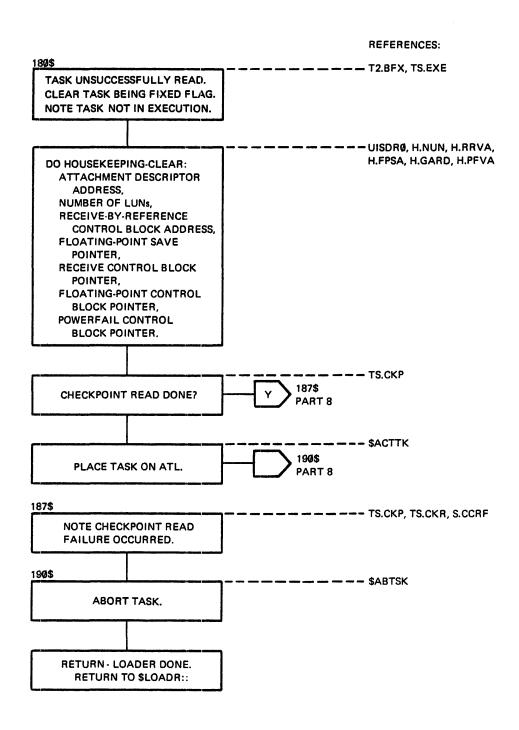
Figure 2-11 Loader Logical Flow Diagram (Part 8 of 8)
