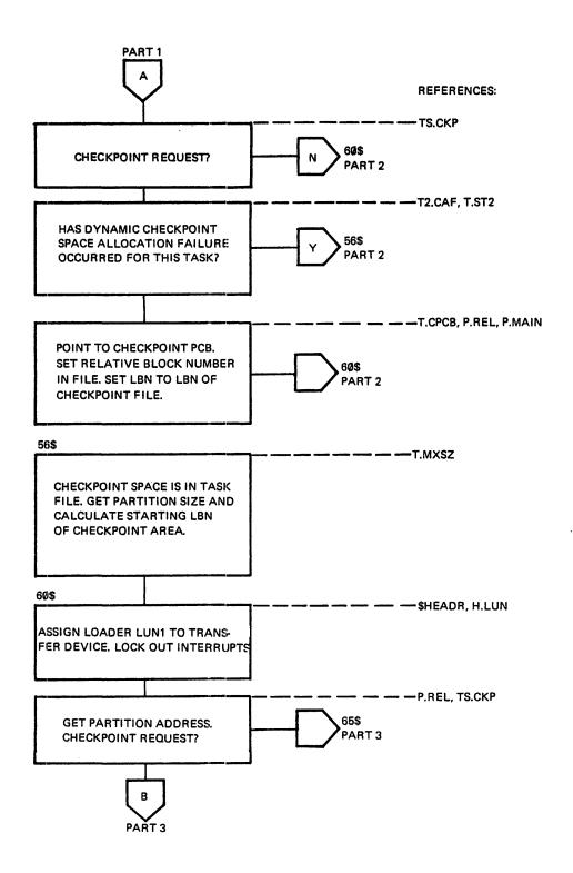
Figure 2-11 Loader Logical Flow Diagram (Part 2 of 8)
