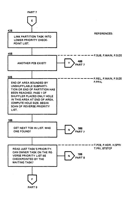
Figure 2-12 Shuffler Logical Flow Diagram (Part 8 of 11)
