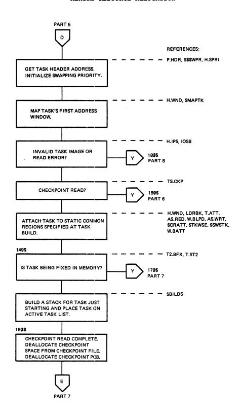
Figure 2-11 Loader Logical Flow Diagram (Part 6 of 8)
