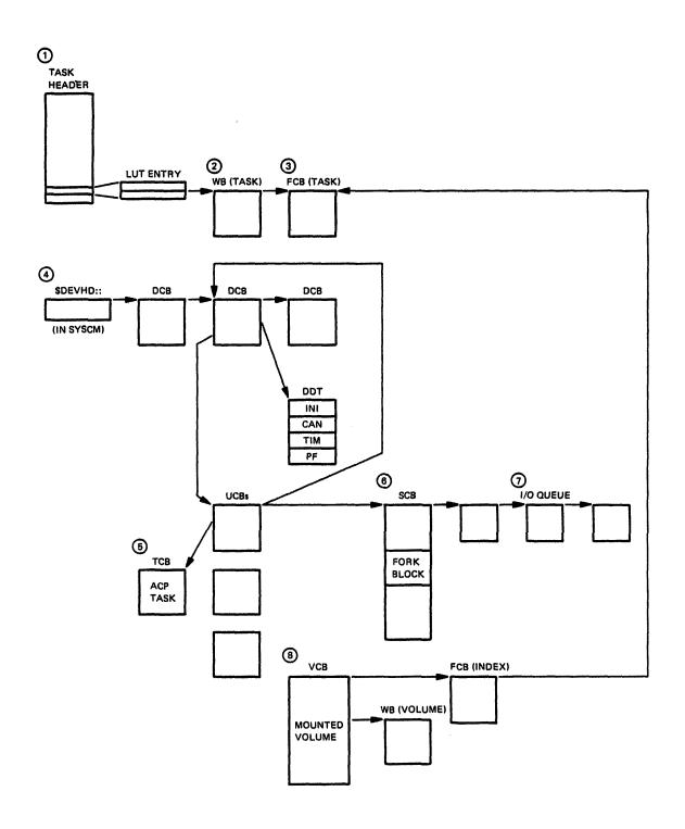
Figure 8-24 I/O Data Structure
