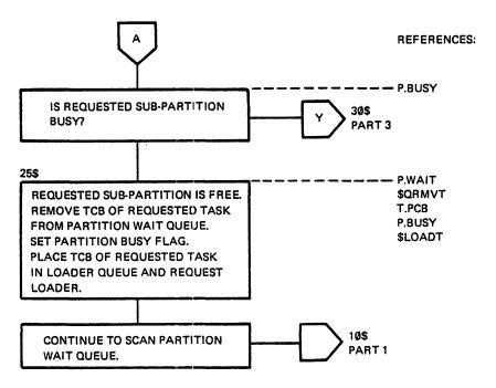
Figure 2-9 \$NXTSK Logical Flow Diagram (Part 2 of 7)
