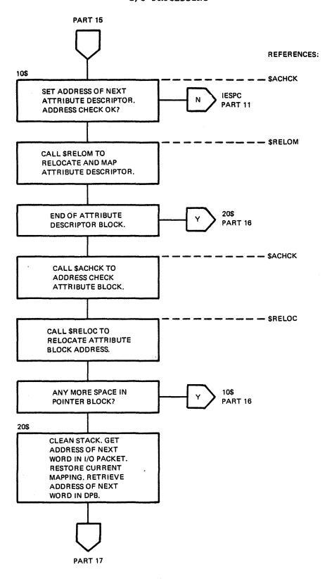
Figure 6-2 QIO Directive Processing (Part 16 of 24)
