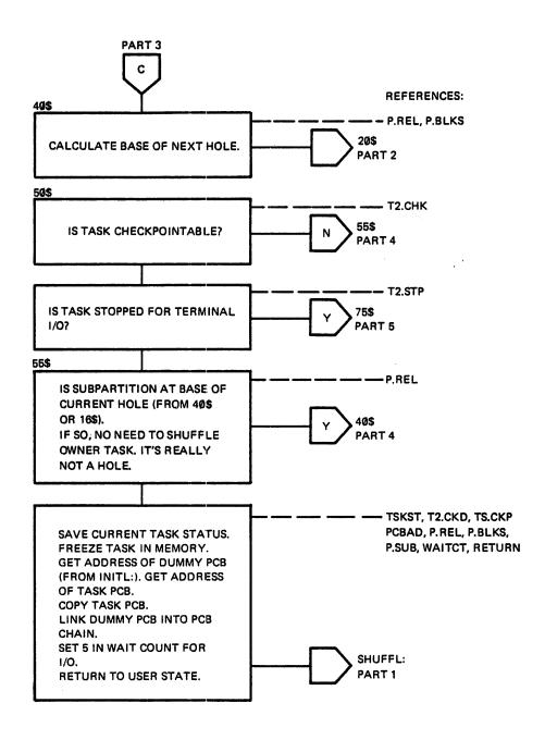
Figure 2-12 Shuffler Logical Flow Diagram (Part 4 of 11)
