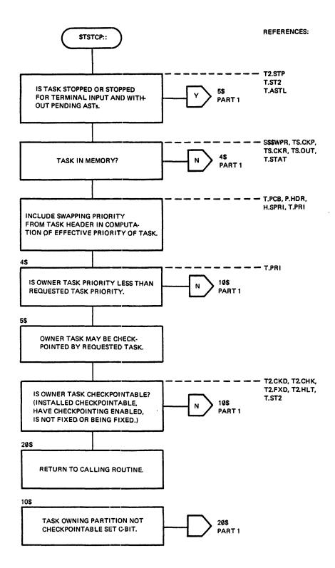
Figure 2-10 \$TSTCP Logical Flow Diagram (Part 1 of 1)
