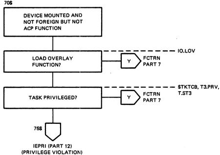
Figure 6-2 QIO Directive Processing (Part 5 of 24)
