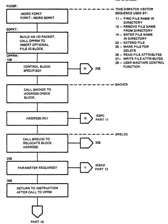
Figure 6-2 QIO Directive Processing (Part 14 of 24)
