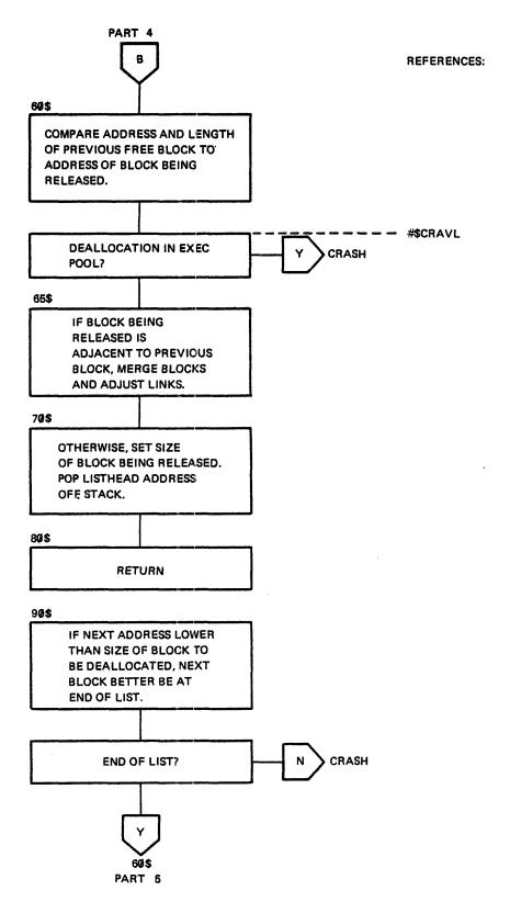
Figure 2-6 \$DECLK-\$DEPKT-\$DEACB Logical Flow Diagram (Part 5 of 5)
