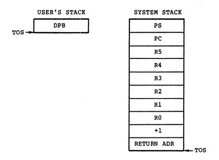
Figure 3-4 Stack State Upon Entry into Directive Processing
