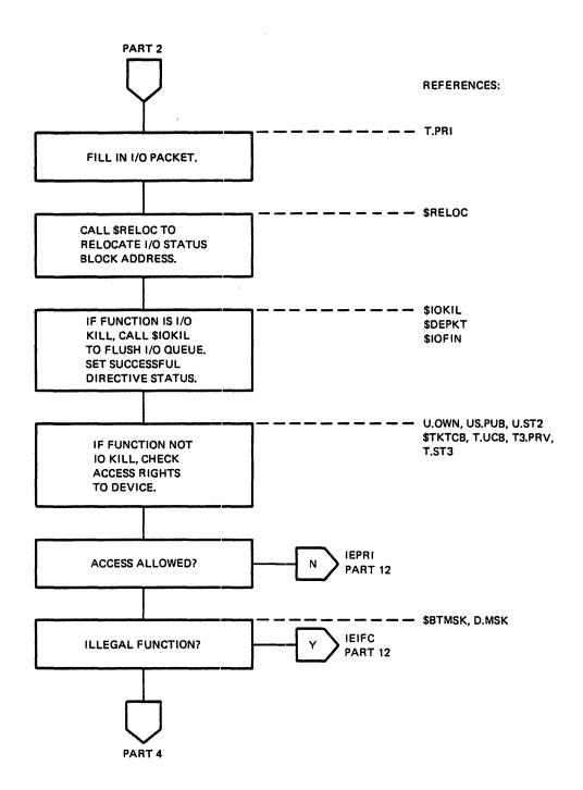
Figure 6-2 QIO Directive Processing (Part 3 of 24)
