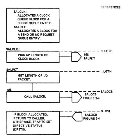
Figure 2-3 \$ALCLK Logical Flow Diagram
