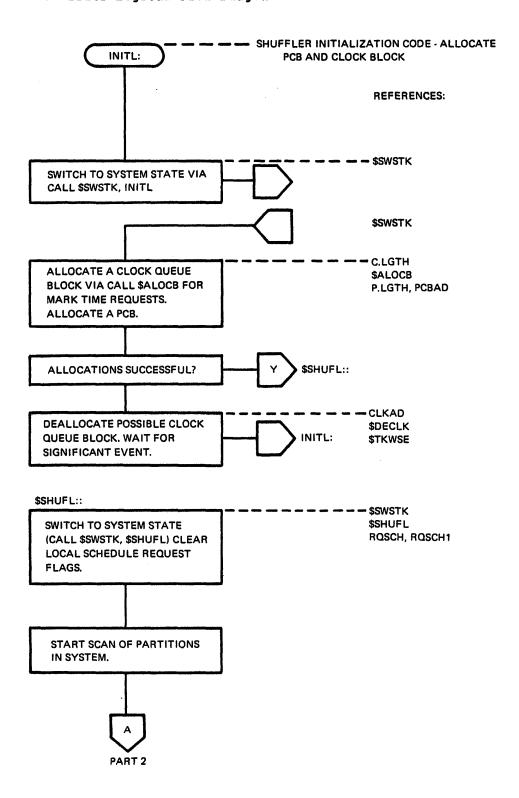
Figure 2-12 Shuffler Logical Flow Diagram (Part 1 of 11)
