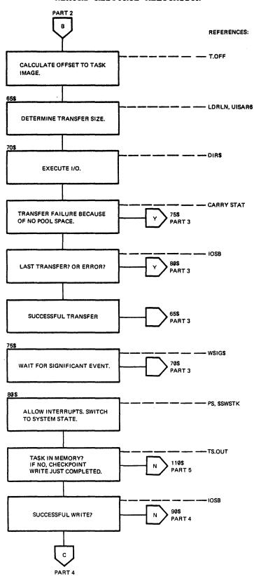
Figure 2-11 Loader Logical Flow Diagram (Part 3 of 8)
