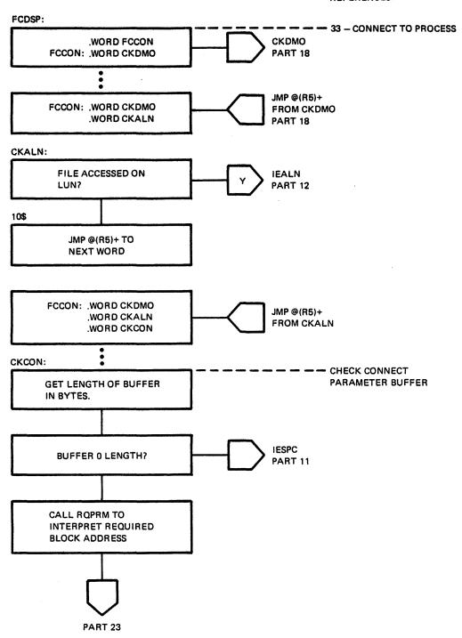
Figure 6-2 QIO Directive Processing (Part 22 of 24)
