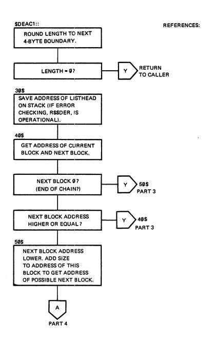
Figure 2-6 \$DECLK-\$DEPKT-\$DEACB Logical Flow Diagram (Part 3 of 5)
