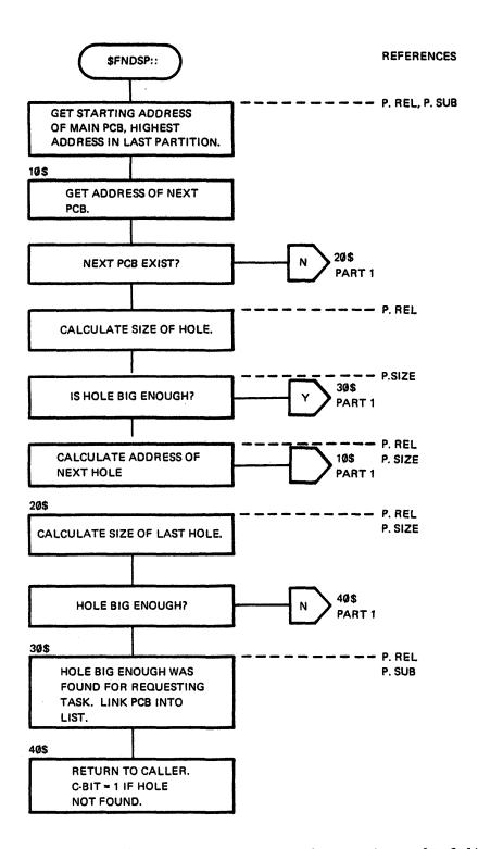
Figure 2-7 \$FNDSP Logical Flow Diagram (Part 1 of 1)
