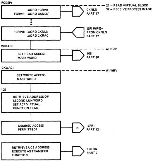
Figure 6-2 QIO Directive Processing (Part 20 of 24)
