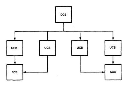
Figure 8-23 I/O Data Structure for Two RKll Disk Controllers
