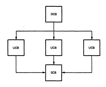
Figure 8-22 RKll Disk I/O Data Structure
