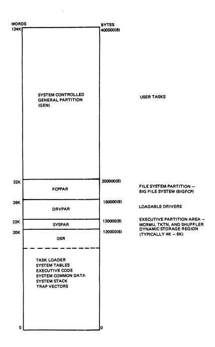
Figure 1-2 Example of a Mapped 124K RSX-11M System
