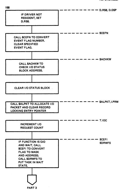
Figure 6-2 QIO Directive Processing (Part 2 of 24)
