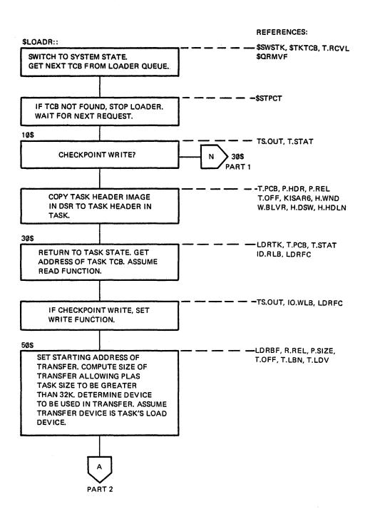
Figure 2-11 Loader Logical Flow Diagram (Part 1 of 8)
