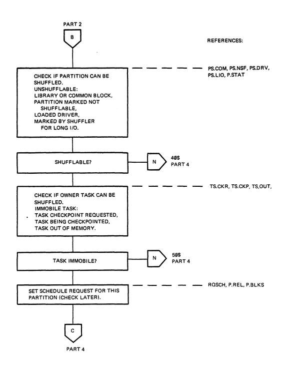
Figure 2-12 Shuffler Logical Flow Diagram (Part 3 of 11)
