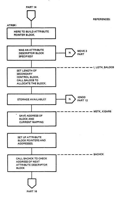
Figure 6-2 QIO Directive Processing (Part 15 of 24)
