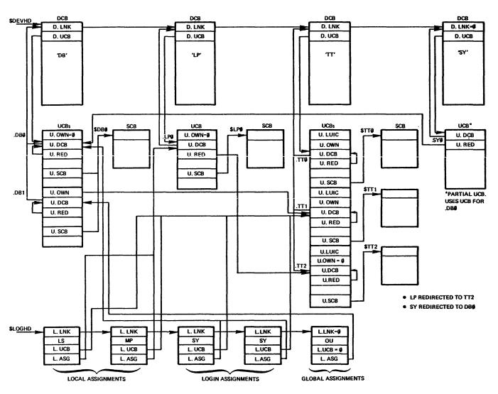
Figure 8-15 Example of DCB, SCB, UCB, LCB Relationship
