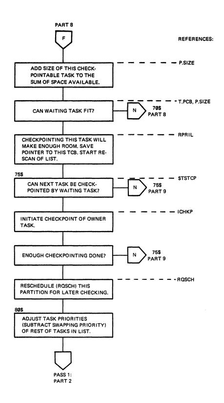
Figure 2-12 Shuffler Logical Flow Diagram (Part 9 of 11)
