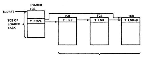
TCBs OF TASKS TO BE LOADED OR ROLLED OUT/IN ARE CHAINED ACCORDING TO THE RUNNING PRIORITY OF THE TASKS IN DESCENDING ORDER.
