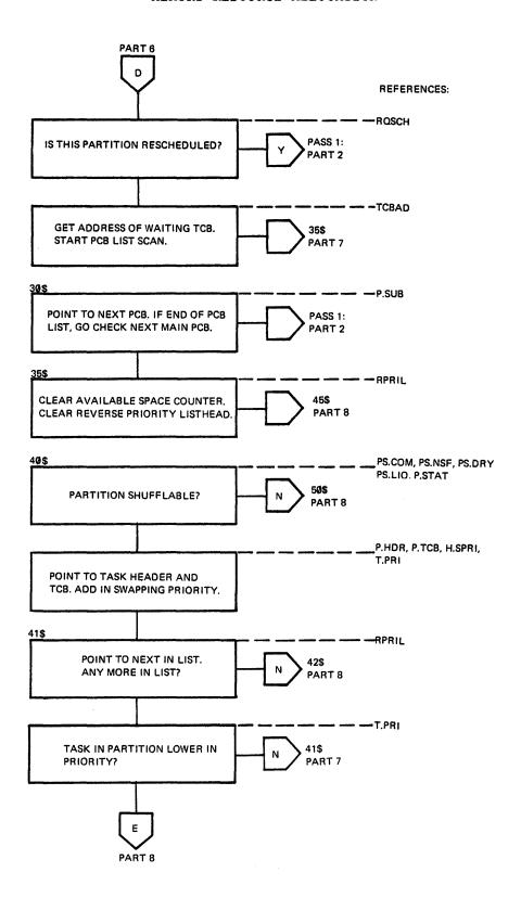
Figure 2-12 Shuffler Logical Flow Diagram (Part 7 of 11)
