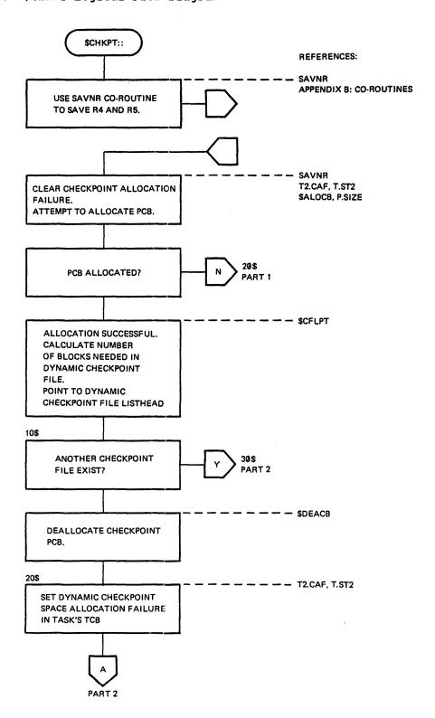
Figure 2-5 \$CHKPT Logical Flow Diagram (Part 1 of 2)
