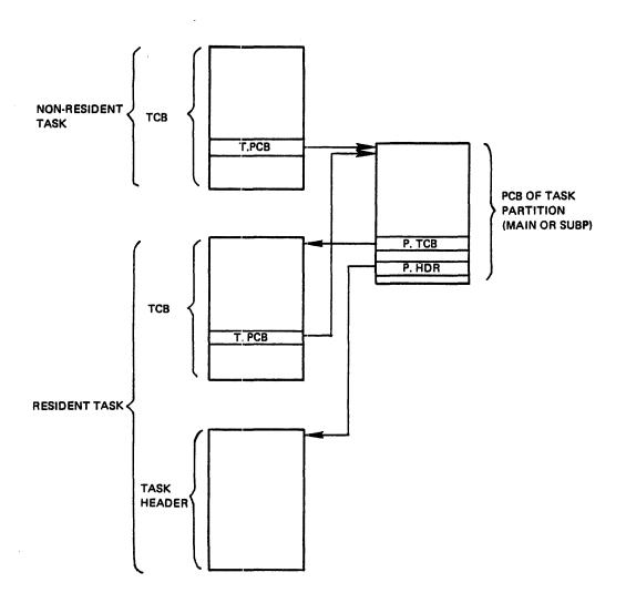
Figure 8-7 Simplified User-Controlled Partition TCB, Task Header, and PCB Relationship
