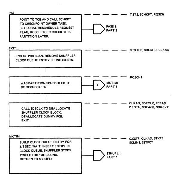
Figure 2-12 Shuffler Logical Flow Diagram (Part 5 of 11)
