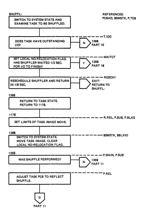
Figure 2-12 Shuffler Logical Flow Diagram (Part 10 of 11)
