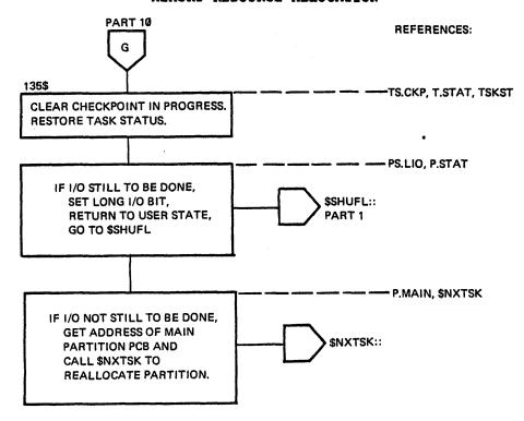
Figure 2-12 Shuffler Logical Flow Diagram (Part 11 of 11)
