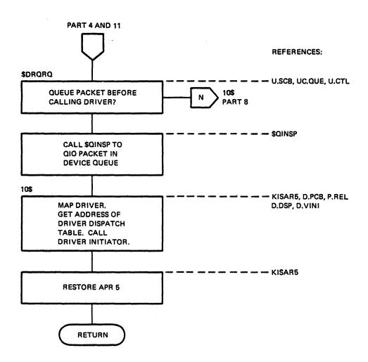
Figure 6-2 QIO Directive Processing (Part 8 of 24)
