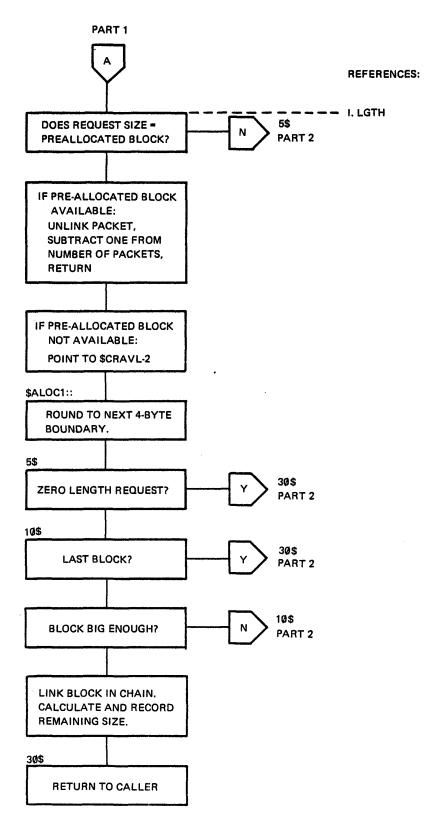
Figure 2-4 \$ALOCB Logical Flow Diagram (Part 2 of 2)
