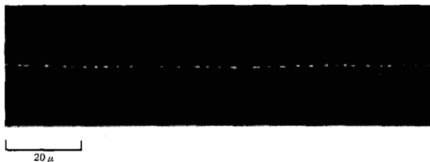
Figure 14 Bitter pattern of a Bloch wall in a 1000 Å film with Néel lines visible as bright spots. A hard direction dc field was applied of about \frac{1}{4} H_k .
